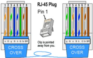
CROSSOVER CABLES - The purpose of a Crossover Ethernet cable is to directly connect one computer to another computer (or device) without going through a router, switch or hub.
